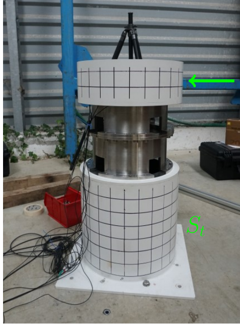
Figure 2.22 – Picture of the set-up used to determine the locations of the accelerometers on the skin element. The green arrow indicates the position at which the skin element was impacted.
