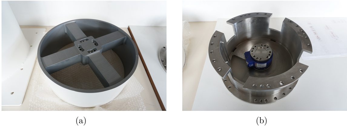
Figure 2.6 – (a) Skin and (b) backbone element of a section. The load cell is mounted on the inner part of the section.
