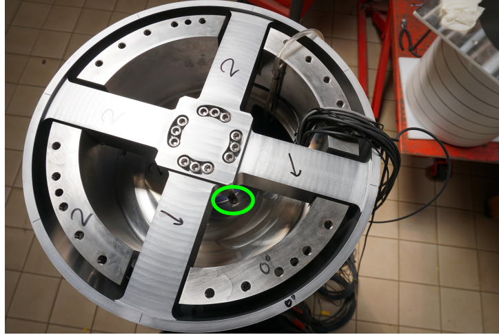
Figure 2.15 – Accelerometer mounted on the skin element of the second section.
