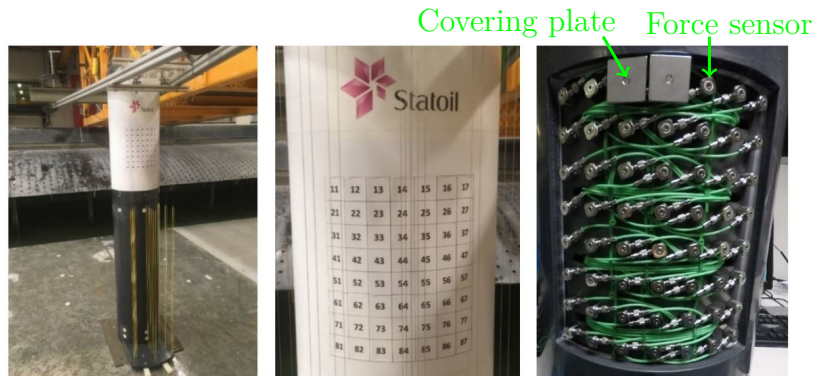
Figure 1.16 – Description of the cylinder used in the experiments of Lian 2018. From left to right, the pictures display the cylinder fixed in the basin, the force transducers numbering and the force transducers and steel plates.
