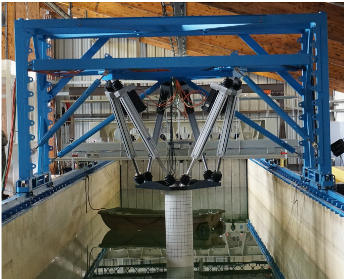
FIGURE 1: OVERVIEW OF THE CYLINDER, THE HEXAPOD AND THE FLUME.
