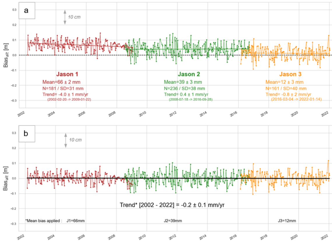
Figure 9. (a) Altimeter bias time series at the comparison point for Jason-1 (red), Jason-2 (green), and Jason-3 (orange) track 162. (b) Altimeter bias time series after applying mean biases found in this study (i.e. -66 mm for J1, -39 mm for J2 and -12 mm for J3). The black line represents the resulting trend computed over the whole Jason period (2002–2022).
