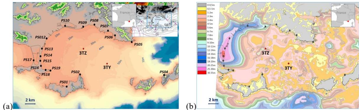
Fig.1. The experiment site, namely the Rade d'Hyères in the Mediterranean Sea (south-eastern part of France): (a) bathymetry, (b) 3D map of the sediment thickness. The two locations, labeled 3TY and 3TZ, are the locations where the UXO were detonated during the campaign of December 2018. The locations of the temporary seismological stations deployed along the shore are labeled PS01-PS19.
