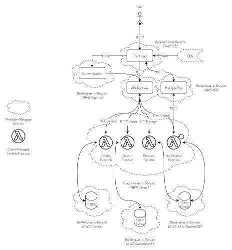
Fig. 5 Fictional reference architecture for a serverless e-commerce web application deployed in the Amazon Web Services ecosystem
