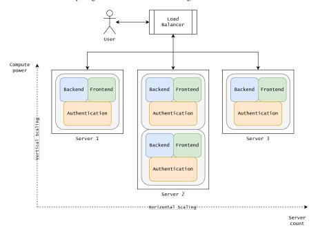
Fig. 3 Scaling out a monolith-architectured application requires replicating the monolith on multiple servers
