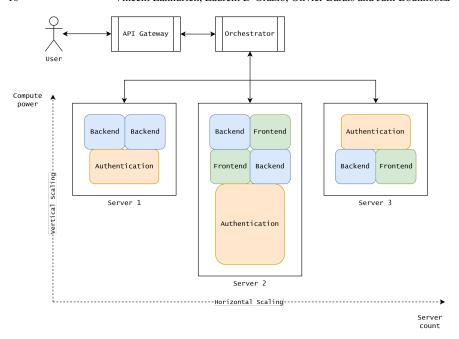
Fig. 4 Scaling out a microservices-architectured application allows distributing and replicating each microservice independently
