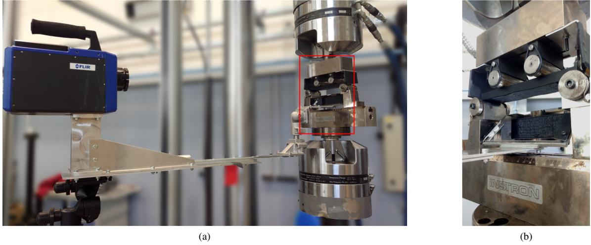
FIGURE 3 – Image of the four-point bending test fixture and the infrared camera (a) and zoom showing the mounted sample and the infrared mirror (b)
