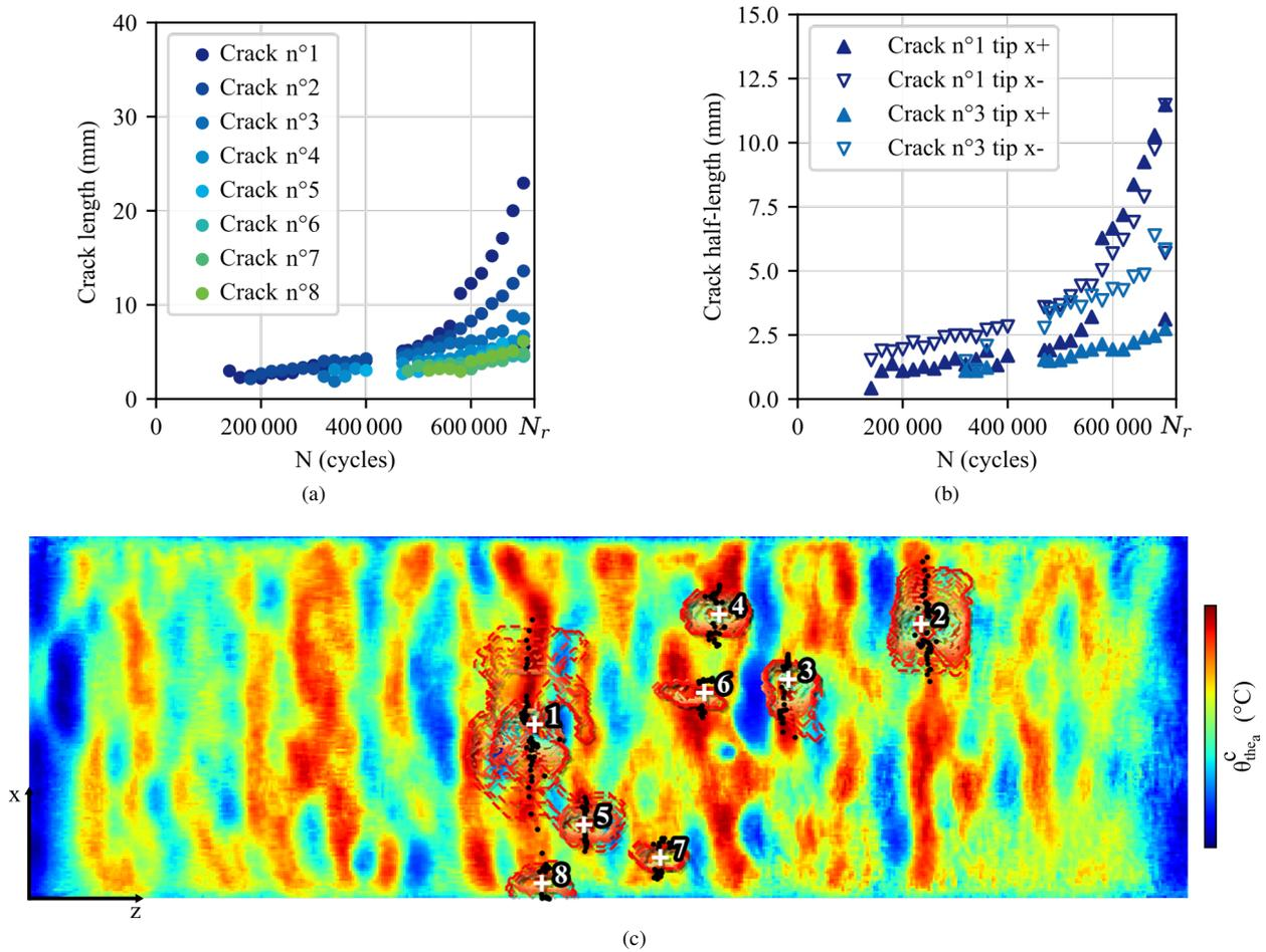
FIGURE 12 – Crack propagation curves in full crack length (a) and half crack length (b) and crack initiation sites, crack tips positions and binary crack shapes on the initial  $\theta_{the_a}^c$  field (c)
