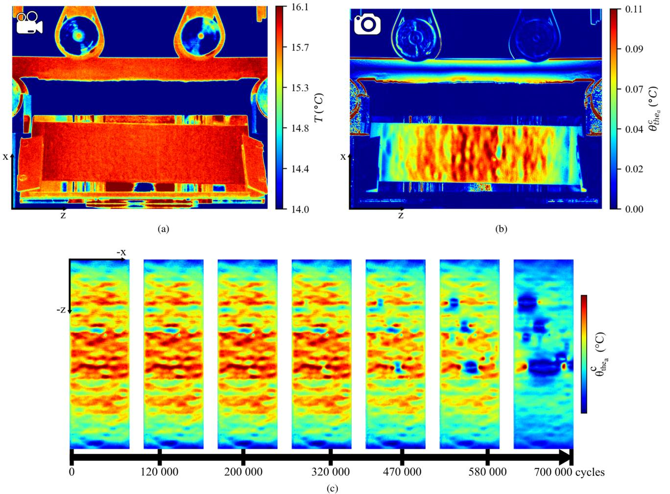
FIGURE 5 – Frame of an infrared film of *SPII* (a), field of the temperature amplitude  $\theta_{the_a}^c$  linked to the thermoelastic coupling of the corresponding infrared film as determined by the lock-in method (b) and evolution of the temperature amplitude  $\theta_{the_a}^c$  field on the rough surface of sample *SPII* during its fatigue test (c)
