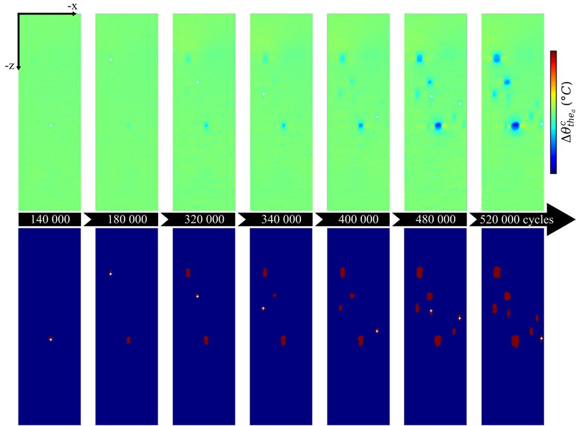
FIGURE 7 – Evolution of the differential of temperature amplitude  $\Delta\theta_{the_a}^c$  field on the rough surface of sample *SPII* with the corresponding binary images (initiation sites shown in white)
