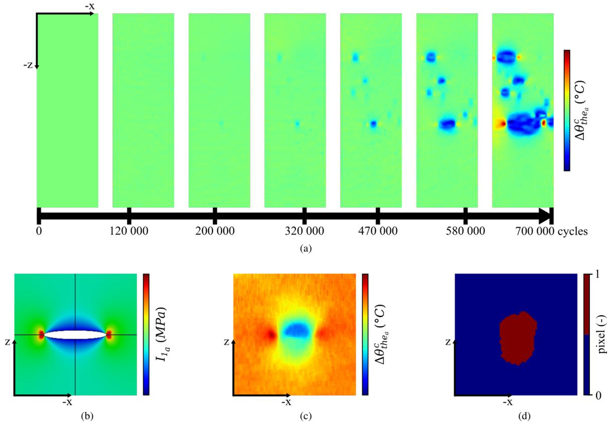
FIGURE 6 – Evolution of the differential of temperature amplitude  $\Delta\theta_{the_a}^c$  field on the rough surface of sample *SPII* during its fatigue test (a), illustration of the  $I_{1_a}$  field around a fictive 2D crack in mode I (b), experimental  $\Delta\theta_{the_a}^c$  field around a crack in a rough WAAM surface (c) and corresponding binary image after thresholding (d)
