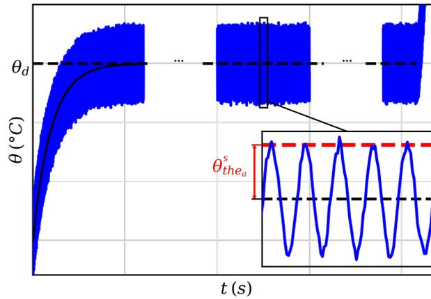
FIGURE 4 – Schematic illustration of the sample's surface mean temperature variation  $\theta$  during a complete fatigue test, composed of an intrinsic dissipation contribution  $\theta_d$  and a thermoelastic contribution  $\theta_{the_a}^s$
