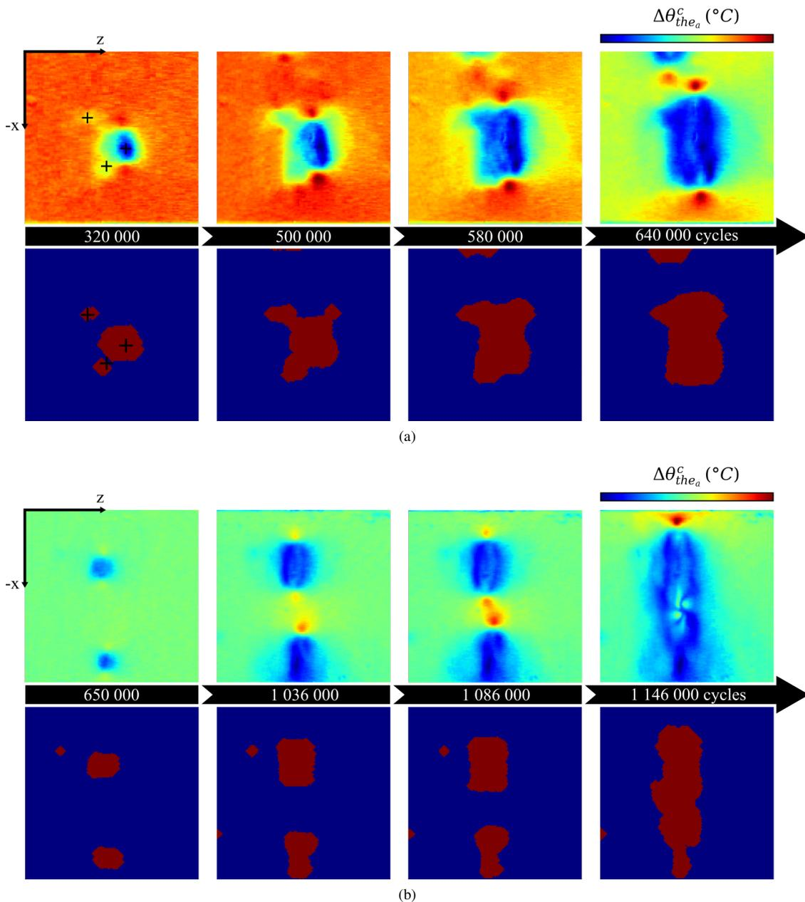
FIGURE 9 – Crack obscuration phenomenon demonstrated on sample *SPIII*: of the three cracks visible on the images, only one propagates throughout the whole fatigue life, as the two smaller cracks are obscured (a); and coalescence phenomenon on sample *SPIV*: two cracks initiate at a close  $z$  coordinate and propagate towards each other until meeting and merging (b)
