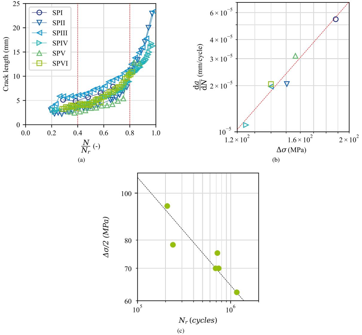
FIGURE 13 – Propagation curves in normalized number of cycles for sample *SPI* to *SPVI* (a), corresponding propagation speed between 40% and 80% of the total fatigue life (b) and fatigue tests results of rough WAAM samples *SPI* to *SPVI* (c)
