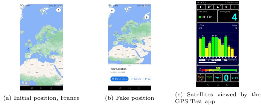
Figure 4: Receiving fake GPS signals
