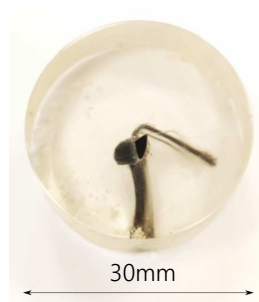
Figure 8. Sample K cast in resin ready for digital microscope observations
