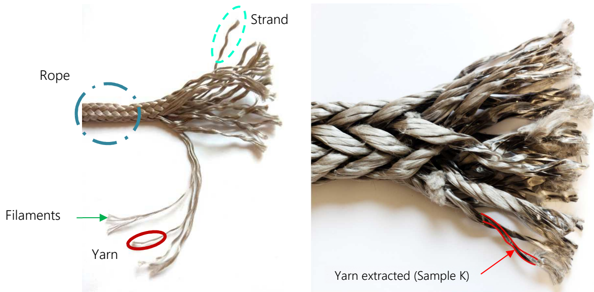
Figure 2.a. The different scales of the Dyneema™ SK99 braided rope of the study with a 4mm diameter, coating and a Mean Breaking Load (MBL) of 14.7kN.
