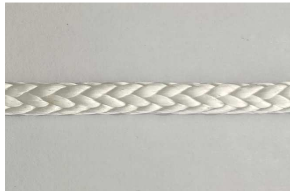
Figure 3. b. Uncoated HMPE fiber rope, 4mm diameter
