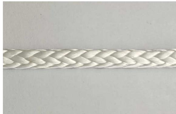
Figure 3. a. Coated HMPE fiber rope, 4mm diameter
