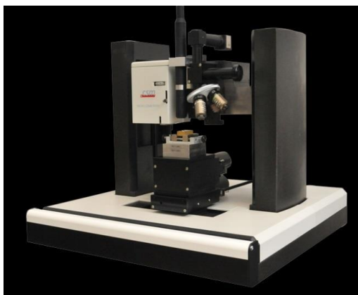
Figure 1. Indentation machine and representative plot of the load versus displacement.
