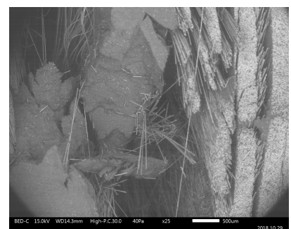
Damaged sample at 4 bar
