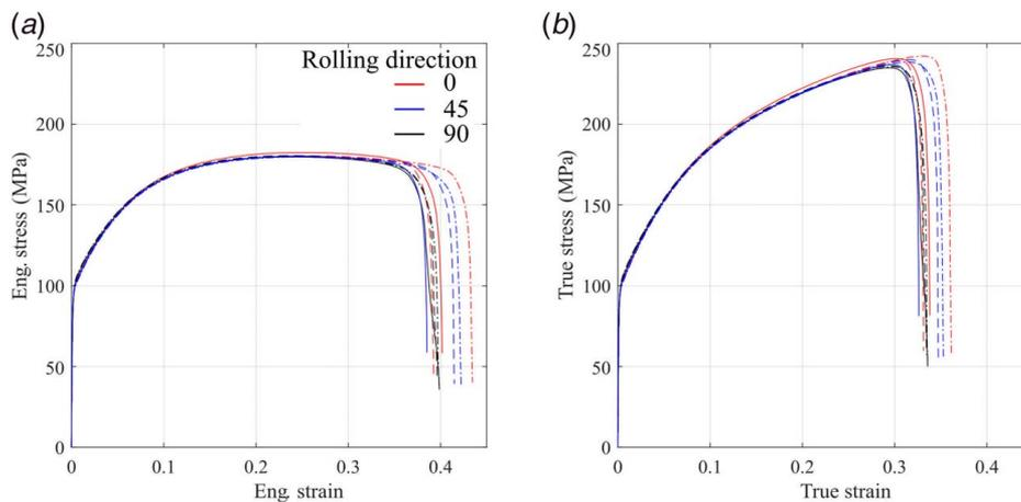
**Fig. 3 (a) Engineering and (b) true tensile mechanical properties of high-purity niobium polycrystalline sheets at a nominal strain rate of  $\sim 1.08 \times 10^{-3} \text{ s}^{-1}$  for different rolling directions. Dashed and dash-dotted lines are repetitions of tests with the same rolling direction.**
