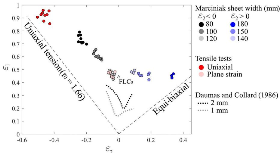
**Fig. 5 Forming limit curve of high-purity niobium for sheets aligned with the rolling direction parallel to the major strain axis and an approximated value of FLC<sub>0</sub> for pure plane-strain deformation ( $n = 0.236$  and  $m = 0.112$ ). The experimental FLCs measured by Daumas and Collard [11] for niobium sheets with thicknesses of 1 and 2 mm are also presented for comparison with this study.**
