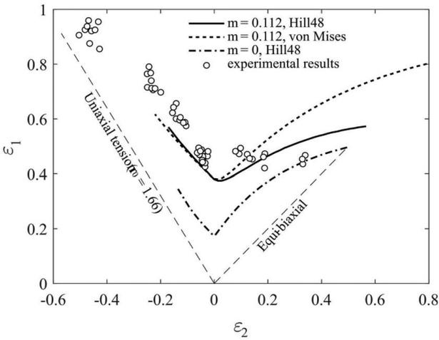
**Fig. 6 Comparison between FLCs derived from the two-zone model and the experimental necking strains. The reference curve ( $m=0.112$ , Hill 48) has been obtained with the material parameters given in Table 3 and an imperfection amplitude  $\xi=0.5\%$ . The FLCs corresponding to an isotropic von Mises material ( $F=G=H=0.5$  and  $N=1.5$ ) and a rate-insensitive material ( $m=0$ ) are also presented. The principal initial strain rate is  $\dot{F}_{11}=10^{-3}\text{ s}^{-1}$ .**
