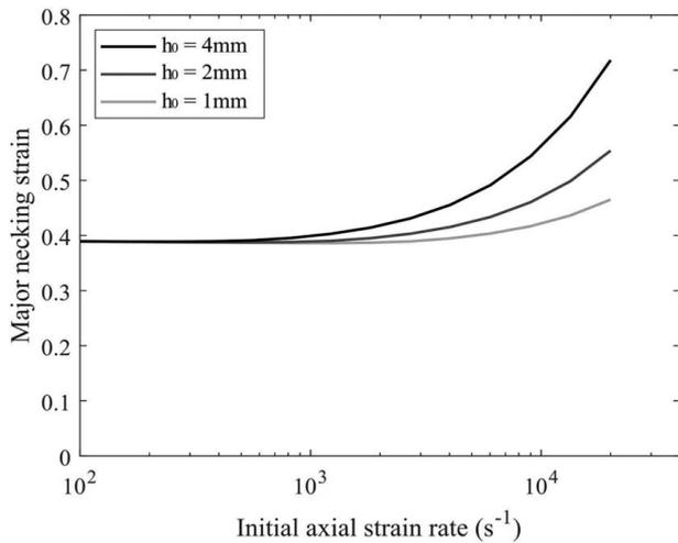
**Fig. 7 Evolution of the major necking strain as a function of the initial axial strain rate  $\dot{F}_{11}$  for several values of initial sheet thickness  $h_0$ . The loading conditions corresponds to plane-strain stretching ( $F_{22}=0$ ) and the imperfection amplitude is  $\xi=0.5\%$ .**
