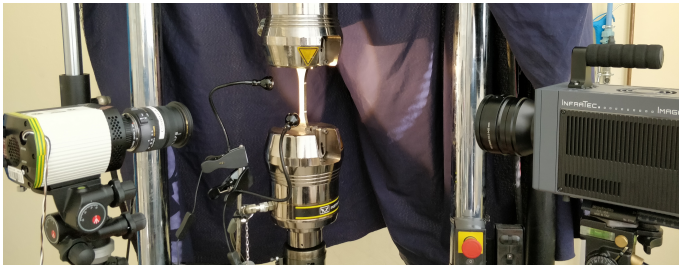
Fig. 6 Experimental setup combining infrared imaging with digital image correlation.
