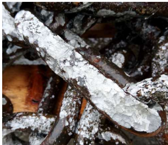
Fig. 2. Bio-corroded link after high pressure cleaning
