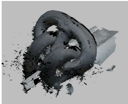
Fig. 4. Scan of stud link without processing, with the holding support and the adjacent links.
