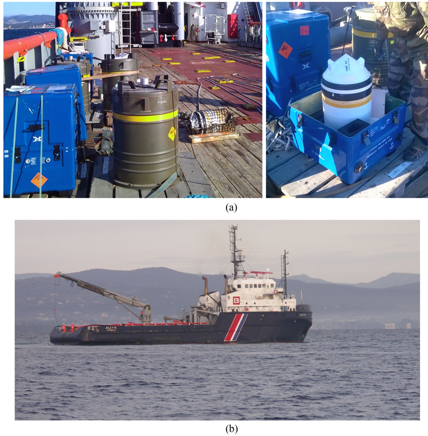
Fig. 4. (a) Charges of 200-kg (left) and 80-kg (right) TNT-equivalent stacked in a container, before being dipped to water. (b) Ship named BSAD Ailette that transported the charges to the locations of their countermining.
