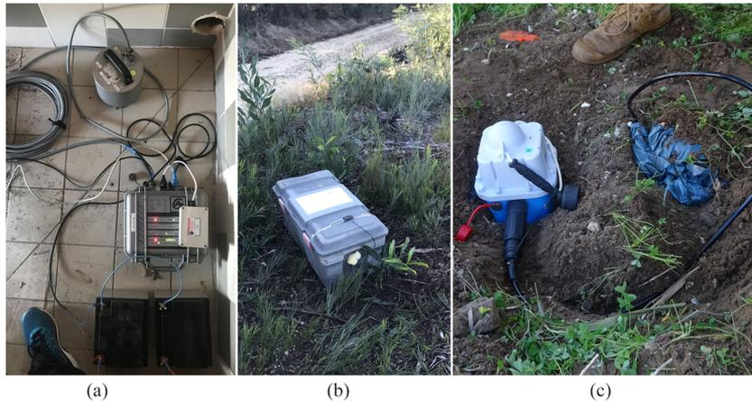
Fig. 6. (a) Broadband sensor and a digitizer installed in a small room at the location labeled PS12 in Fig. 1. (b) and (c) When the instruments were installed outside, the sensors were buried, and all the associated parts (digitizer, disk, and batteries) were placed in a plastic box, as illustrated (b) for the sensor located at PS07 in Fig. 1.
