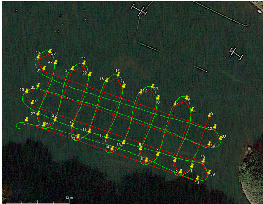
FIGURE 10 | The real boustrophedon track (in green) with the desired waypoints (in yellow, connected by red lines). Short legs are approximately 20 m and long ones are 70 m.
