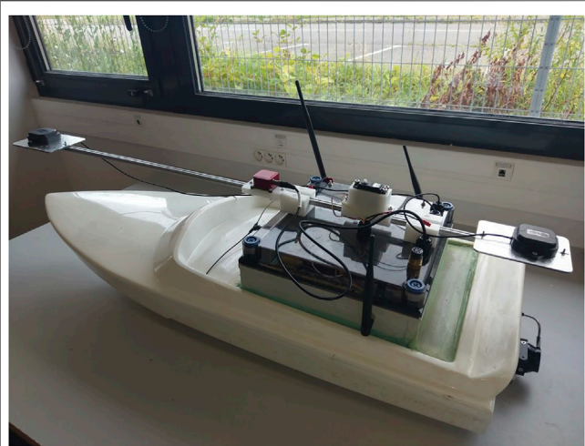
FIGURE 1 | Autonomous boat with an interval-based inertial navigation system (INS).
