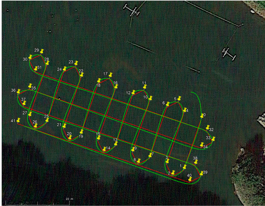
FIGURE 9 | The simulated boustrophedon track (in green) with the desired waypoints (in yellow, connected by red lines). Short legs are approximately 20 m and long ones are 70 m.
