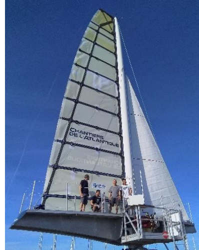
Figure 1 Jib Sea prototype at 1:5 scale.
