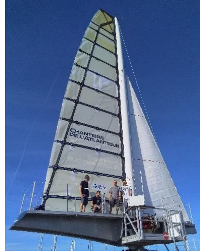
Figure 1 Jib Sea prototype at 1:5 scale.
