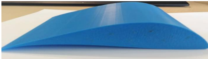
Figure 18. Experimental 3D printed NTSXX20 Hydrofoil
