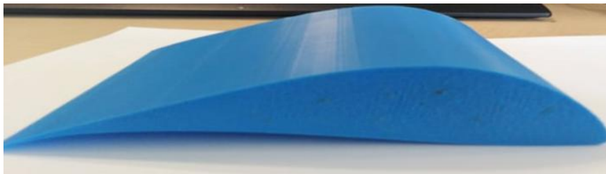
Figure 18. Experimental 3D printed NTSXX20 Hydrofoil
