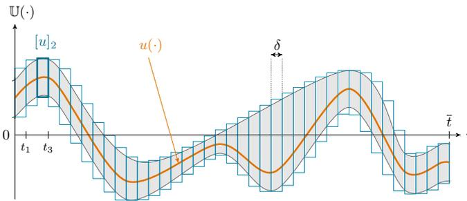
Figure 2: Illustration of a tube  $\mathbb{U}(\cdot)$  made of slices. This representation can be used in order to reliably enclose sets of trajectories. For instance, the thick blue box depicts the  $[u]_{k=2}$  slice containing the feasible values for  $u(t)$ ,  $t \in [t_2, t_3]$ .
