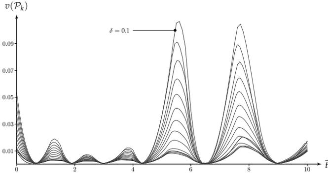
Figure 5: Area of each 2d polygon  $\mathcal{P}_k$  computed with several time steps  $\delta = 0.1 \dots 0.0001$ . The smallest polygons correspond to the measurement times given in Table 1. We observe that the polygonal enclosure rapidly converges towards the exact envelop, corresponding to an infinitely small time step  $\delta$ . This is also illustrated by Figure 6.
