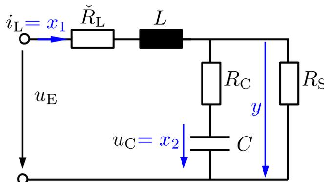
Figure 2. Simplified model of an electrical circuit.
