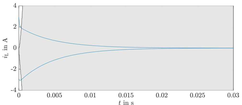
**Figure 5.** Comparison of the presented method relying on cooperativity in blue and a state-of-the-art Taylor series prediction in gray for the state variable  $i_L$ .
