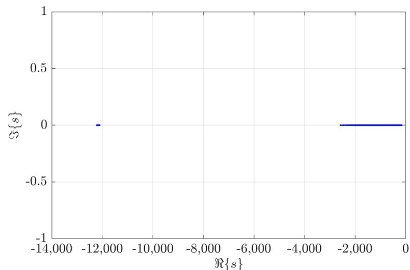
Figure 4. Distribution of eigenvalues for the controlled system.
