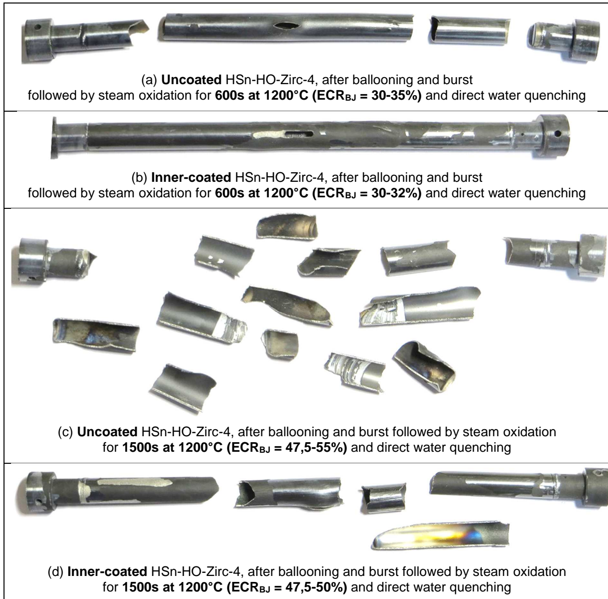
Figure 20 - Visual aspects of uncoated and inner-coated HSn-HO-Zirc-4 clad segments that have experienced internal pressure ballooning and burst temperature ramp tests and then subsequent HT steam oxidation and direct water quenching down to RT
