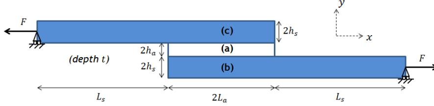
Figure 1: Two-dimensional representation of the single-lap joint
