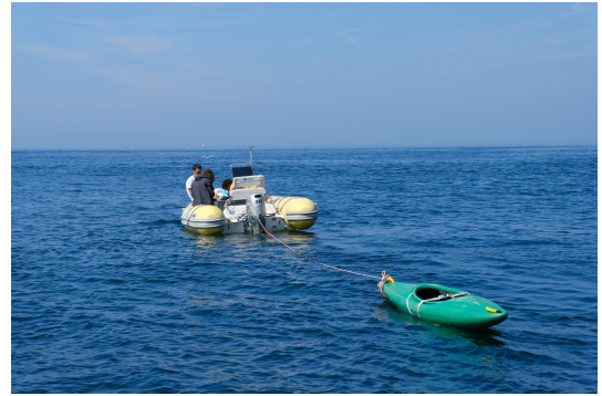
Fig. 2. Boatbot towing a magnetometer
