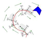
Fig. 10. Since a implies an internal collision and c corresponds to a collision with the polygon, a, c are not in the follow set  $\mathbb{Y}$
