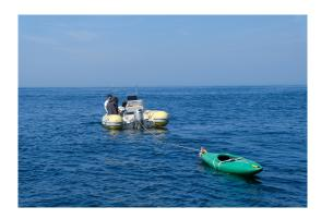
Fig. 2. Boatbot towing a magnetometer
