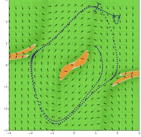
Fig. 12. The green area corresponds to the follow set associated with an internal collision. In the orange area, the controller will lead to a state with an angle  $x_4 - x_3$  too strong and the non-collision constraint will be violated. This Figure has been obtained in 2 minutes.
