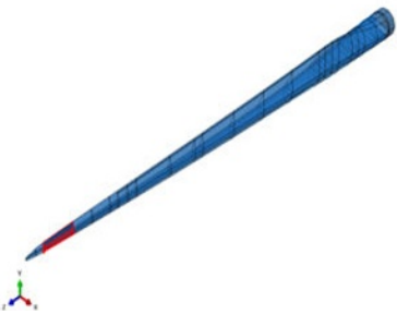
Figure 4: Iced wind turbine blade
