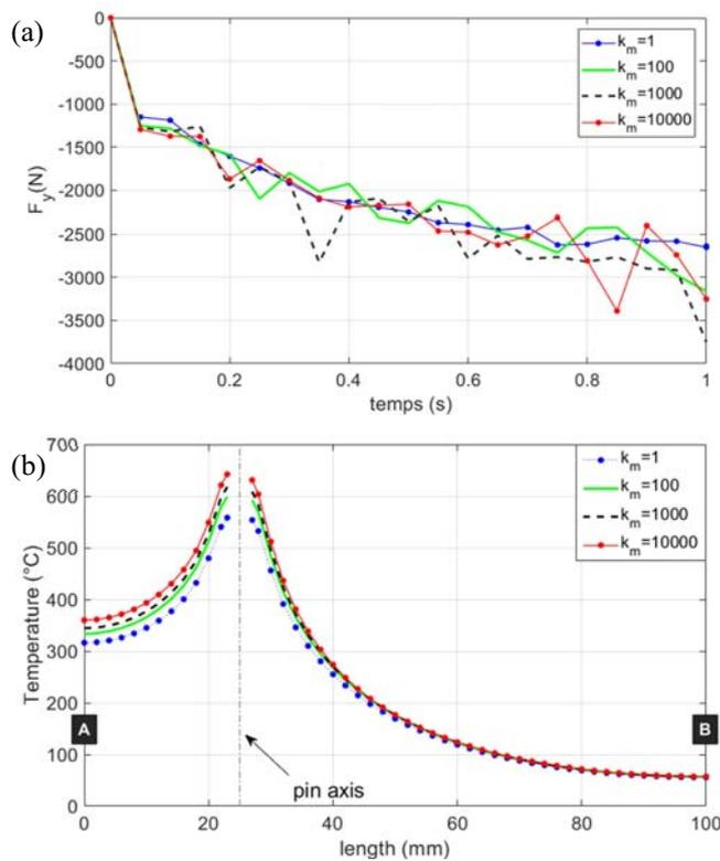
**Figure 4.** Effect of the mass scaling strategy on the down force and the temperature distribution field. (a) down force  $F_y$  evolution during the plunging step with respect to the mass scale factor  $\kappa_m$ ; (b) the distribution of the temperature field on the AB path with respect to the mass scale factor  $\kappa_m$
