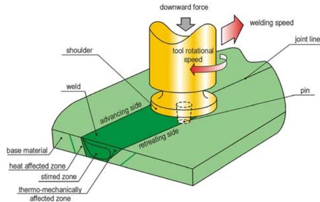
**Figure 1.** A scheme of the FSW process [3].
