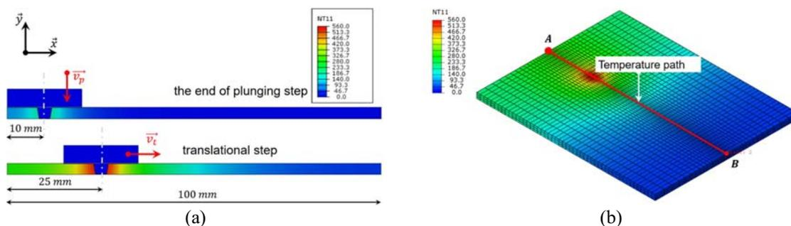
**Figure 3.** The mesh and the simulated temperature distribution field during the FSW joining process. (a) the temperature field in the Z symmetry plane of the FSW joint, at the end of plunging step and during translational step for  $\kappa_m = 1$  (not mass scaling); (b) the temperature field distribution during the translational step. The red line represents the path used to plot the temperature (here  $\kappa_m=1$ ).
