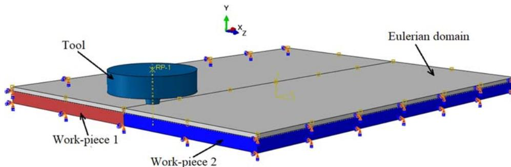
**Figure 2.** ABAQUS FEM model of the FSW process.
