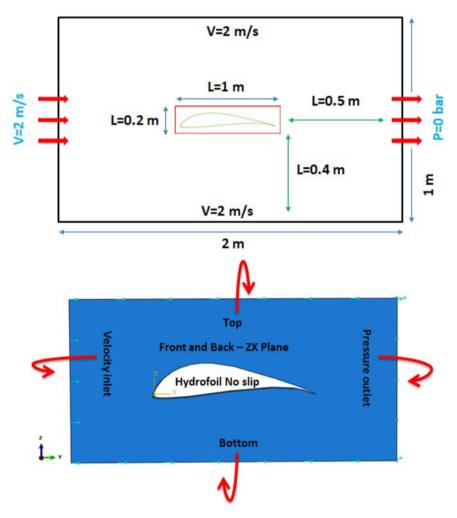
Fig. 13. Schematic diagram of applied boundary conditions in the domain.
