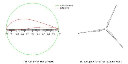
Fig. 11. Design of hydrofoil from the QBlade BEM results.
