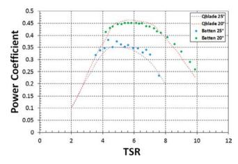
**Fig. 6.** Comparison of performance curves from the QBlade BEM results and experimental data for the Bahaj et al. [23].
