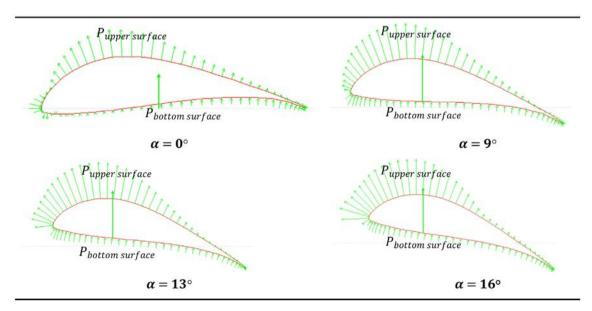
Fig. 10. Schematic representation of lift forces generated in a hydrofoil.
