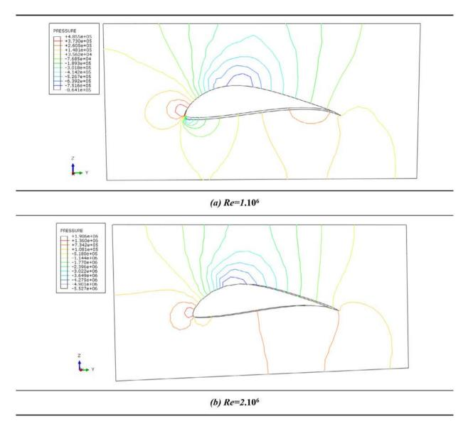
Fig. 17. Pressure distribution (MPa).
