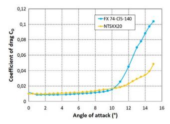
Fig. 8. Variation of the coefficient of drag for NTS-XX20 compared with FX74-CL5-140 at different AOA and Re =  $2.10^{6}$ .
