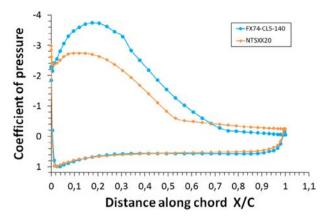
Fig. 9. Pressure coefficient distribution of NTS-XX20 and FX74-CL5-140 at  $\alpha=13^\circ$  and Re =  $2.10^6.$
