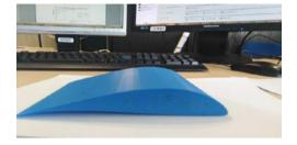
(c)Hydrofoil Manufacture using Additive Manufacturing
