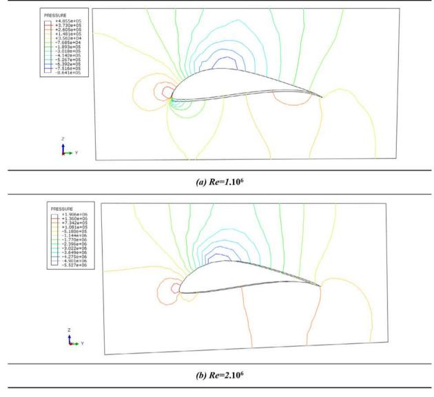
Fig. 17. Pressure distribution (MPa).
