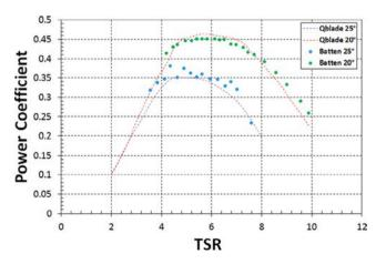
Fig. 6. Comparison of performance curves from the QBlade BEM results and experimental data for the Bahaj et al. [23].
