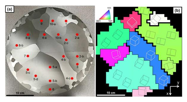
Figure 1: (a) Red points show locations where orientation measurements were performed and (b) normal direction orientation map of the 10 grains with unit cells showing crystal orientation; heavy lines identify coincidence site lattice (CSL) boundaries, and reference x and y directions are labeled.
