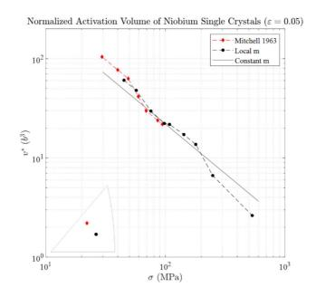
Figure 9: Activation volume as a function of the flow stress at  $\varepsilon = 0.05$ .
