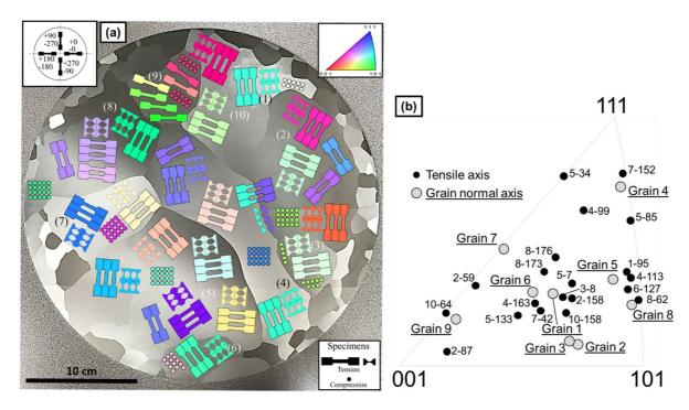
Figure 2: (a) Layout of tensile and cylindrical compression specimens for low and high strain rate tests and (b) inverse pole figure of the tensile axis (black markers) and grain normal axis (grey markers) orientations of all the specimens studied.
