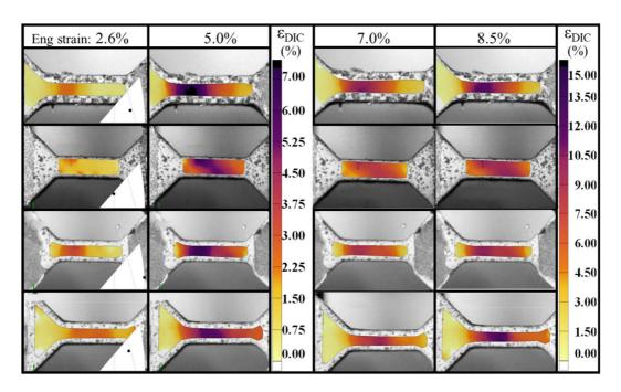
Figure 6: DIC strain maps of four specimens deformed at high strain rates ( $\sim 1000~\text{s}^{-1}$ ) showing strain localization at low engineering strains. The initial tensile direction for each specimen is shown as dots on the inverse pole figure in the lowest strain image of each sample.
