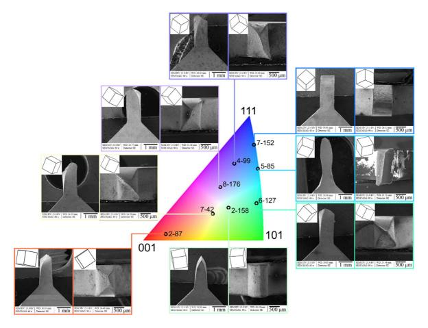
Figure 11: Fracture surface of niobium single crystals deformed at high strain rate in tension for six different orientations with unit cells of undeformed initial orientations normal to each view.
