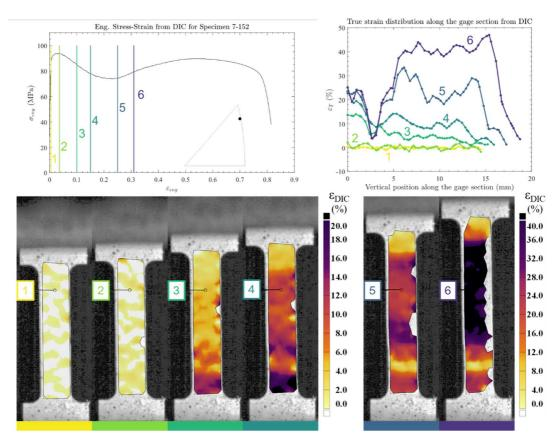
Figure 5: Strain localization of a specimen in the [111] orientation deformed at 1.28x10<sup>-2</sup> s<sup>-1</sup>. (The strain reduction in the neck in 5 and 6 is not physical, but an artefact of the 2D DIC method.)
