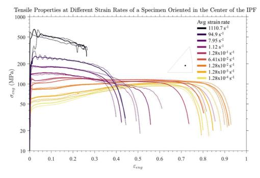
Figure 7: Tensile engineering stress–strain curves with a logarithmic stress scale for strain rates from 1.28x10<sup>-4</sup> to approximately 1000 s<sup>-1</sup> on specimens 2-158 and 3-8 with a crystallographic orientation near the center of the IPF. (Dotted lines are repeat measurements for the same strain rate.)
