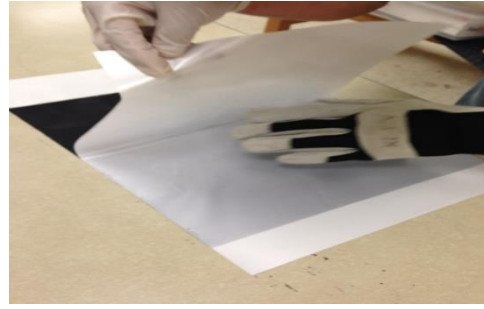
(b) Resin film with nano-additives between two release plies
