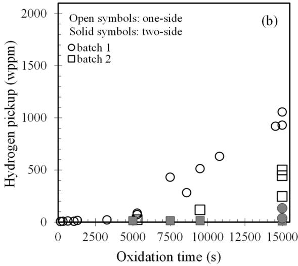
**Fig. 6.** Evolution of (a) the weight gain and (b) the hydrogen pickup (reduced to the cladding outer surface) as a function of the oxidation time for various batches of M5<sub>Framatome</sub> one-sided or two-sided oxidized under steam at 1000°C.
