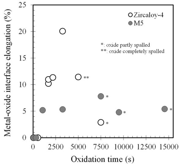
**Fig. 16.** Evolution of the elongation of the metal-oxide interface due to undulation as a function of the oxidation time under steam at 1000°C (one-side oxidation) for Zircaloy-4 (batch 1) and M5<sub>Framatome</sub> (batch 1).
