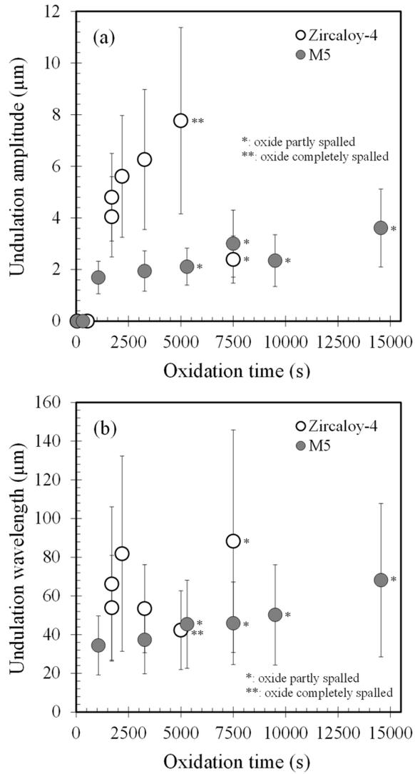
**Fig. 15.** Evolution of (a) the amplitude and (b) the wavelength of the undulations at the metal-oxide interface as a function of the oxidation time under steam at 1000°C (one-side oxidation) for Zircaloy-4 (batch 1) and M5<sub>Framatome</sub> (batch 1).
