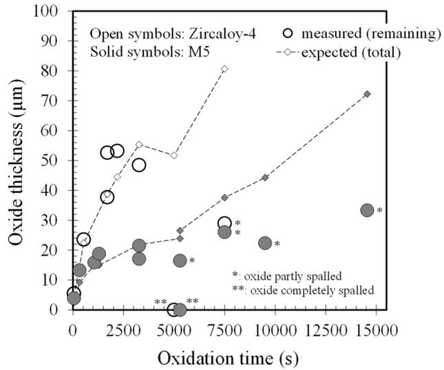
**Fig. 12.** Evolution of the average oxide thickness remaining at the sample surface after quenching and the total oxide thickness expected from the weigh gain (according to the data shown in Fig. 11), as a function of the oxidation time under steam at 1000°C (one-side oxidation) for Zircaloy-4 (batch 1) and M5<sub>Framatome</sub> (batch 1).
