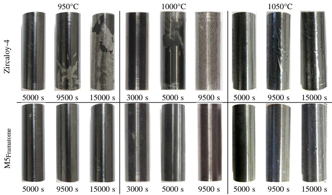
**Fig. 3.** Post-quenching appearance of Zircaloy-4 (batch 2) and M5<sub>Framatome</sub> (batch 2) cladding specimens two-sided oxidized in steam at 950, 1000 and 1050°C.
