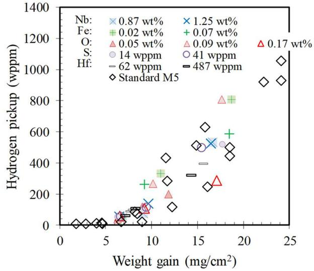
**Fig. 10.** Evolution of the hydrogen pickup as a function of the weight gain at 1000°C (one-side oxidation) for standard M5<sub>Framatome</sub> and materials with chemical compositions (various contents of Nb, Fe, O, S and Hf) around the nominal specifications of M5<sub>Framatome</sub>.
