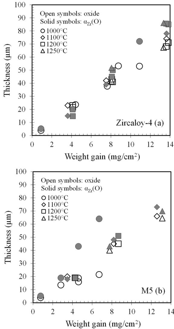
**Fig. 11.** Thicknesses of the oxide layer and the  $\alpha_{\text{Zr}}(\text{O})$  layer as a function of the weight gain at 1000°C (before the onset of breakaway oxidation), 1100°C, 1200°C and 1250°C (one-side oxidation) for (a) Zircaloy-4 (batch 1) and (b) M5<sub>Framatome</sub> (batch 1).
