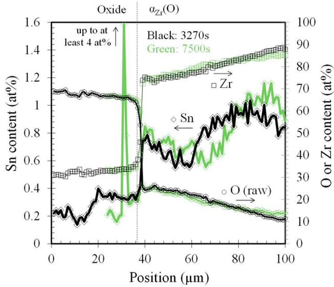
**Fig. 22.** Concentration profiles of tin, zirconium and oxygen (the raw data reported for oxygen overestimate the actual oxygen content values due to surface contamination which was not corrected here) measured by EPMA along the tube radial direction within the oxide and the metallic substrate within Zircaloy-4 (batch 1) samples (one-sided) oxidized for 3270 and 7500 s at 1000°C and water quenched.
