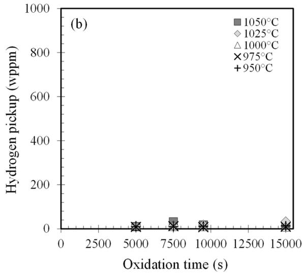
**Fig. 2.** Evolution of (a) the weight gain (the trend lines follow power laws) and (b) the hydrogen pickup (reduced to the cladding outer surface) as a function of the oxidation time under steam at 950, 975, 1000, 1025 and 1050°C (two-side oxidation) for M5<sub>Framatome</sub> (batch 2).
