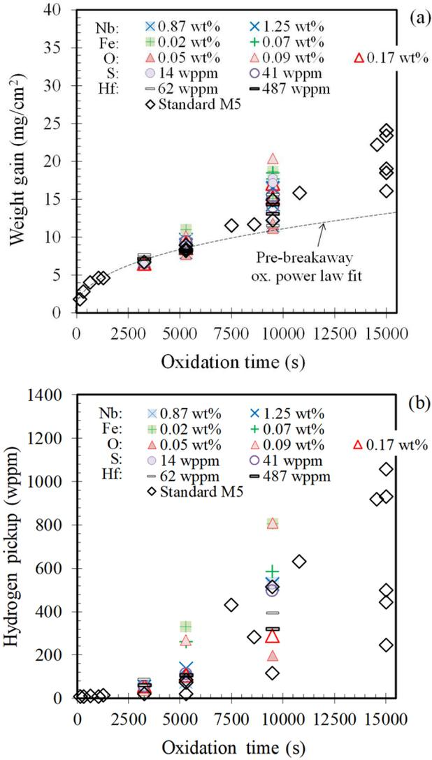
**Fig. 9.** Evolution of (a) the weight gain and (b) the hydrogen pickup as a function of the oxidation time under steam at 1000°C (one-side oxidation) for standard M5<sub>Framatome</sub> (batches 1 and 2) and materials with chemical compositions (various contents of Nb, Fe, O, S and Hf) around the nominal specifications of M5<sub>Framatome</sub>.
