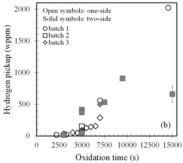
**Fig. 5.** Evolution of (a) the weight gain and (b) the hydrogen pickup (reduced to the cladding outer surface) as a function of the oxidation time for various batches of Zircaloy-4 one-sided or two-sided oxidized under steam at 1000°C.
