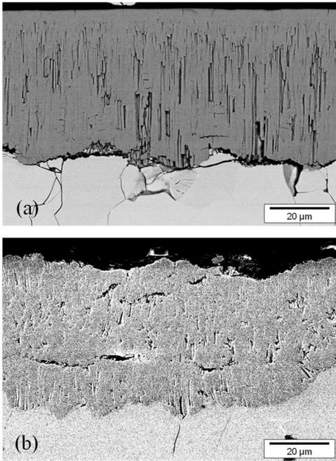
**Fig. 17.** FEG-SEM micrographs of transverse cross-sections of samples one-sided oxidized at 1000°C and water quenched: (a) Zircaloy-4 (batch 1) oxidized 2193s, (b) M5<sub>Framatome</sub> (batch 1) oxidized 14551s (outer part of the oxide layer spalled and therefore not visible).
