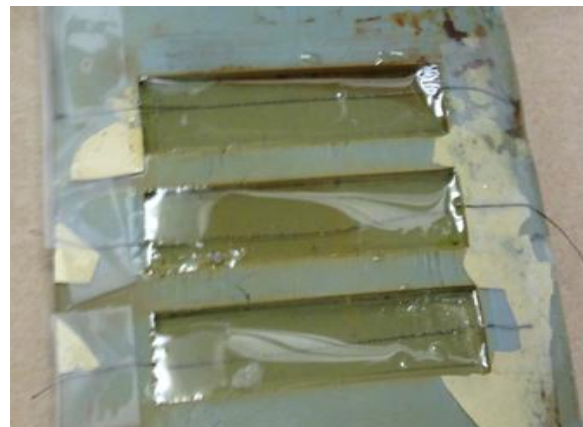
Fig.5. Sensor wire integrated with in the composite specimen
