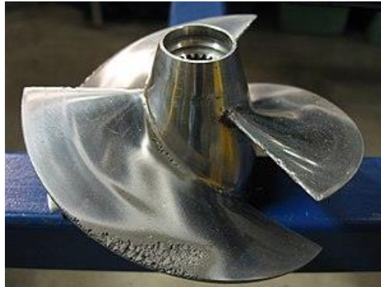
Figure 2. Structural damage due to cavitation.
