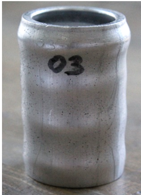
Figure 3: Post-buckled deformed shape of a specimen
