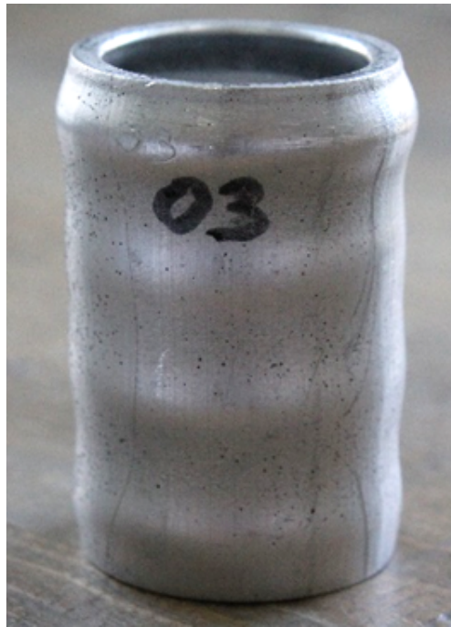
Figure 3: Post-buckled deformed shape of a specimen
