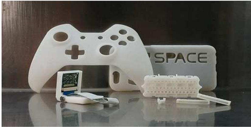
Figure 7: 3D printed system with SLA technology [34].
