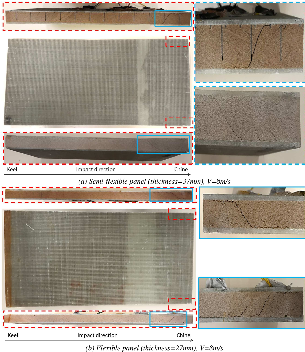
Fig. 5. Damage modes in sandwich panel.
