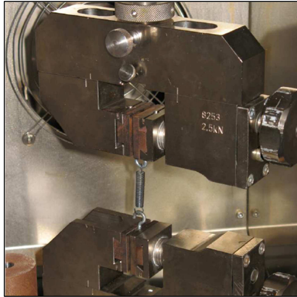
Fig. 8. Experimental set up for detwinning tensile test on the NiTi SMA helical spring.
