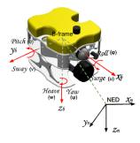
Fig. 1. B-frame and NED-frame of Underwater Vehicles
