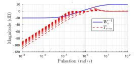
Fig. 4. Bode diagram of  $T_{r \to e}$  for different  $\delta$  values.
