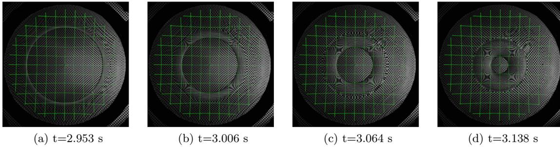
Figure 7: Sequence of images obtained during the water exit of a cone with the draughtboard technique. The diameter of the wetted surface is initially equal to 40 cm.
