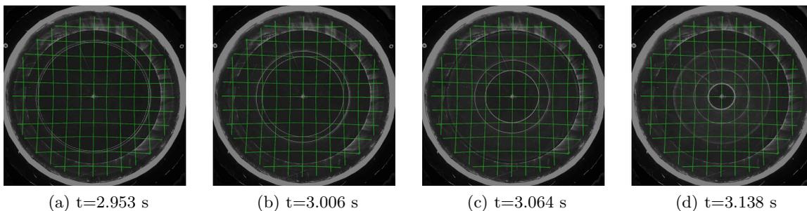
Figure 6: Sequence of images obtained during the water exit of a cone. The diameter of the wetted surface is initially equal to 40 cm.
