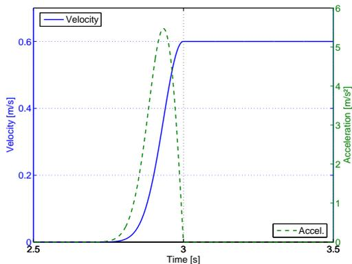
Figure 4: Target velocity and acceleration for the cone water exit
