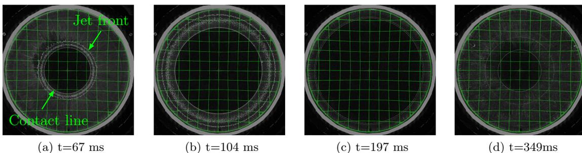
Figure 9: Sequence of images obtained during the water entry (a,b) and exit (c,d) of a cone
