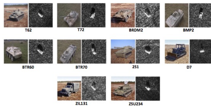
Figure 7. Ten classes of MSTAR database: two tanks (T62 and T72), four armored personnel carriers (BRDM2, BMP2, BTR60 and BTR70), a rocket launcher (2S1), a bulldozer (D7), a truck (ZIL131), and an Air Defence Unit (ZSU234).
