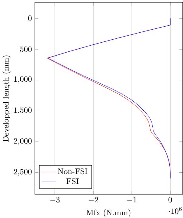
Figure 10: Bending moment distribution along the span
