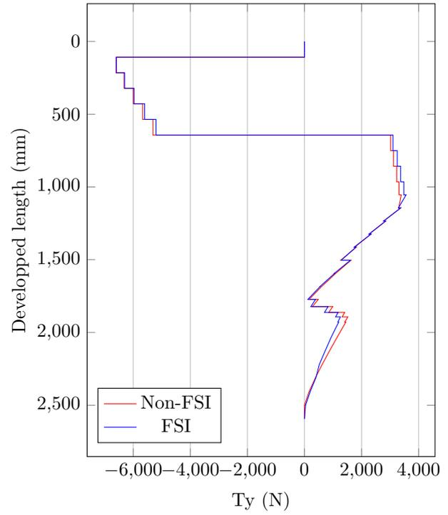
Figure 11: Shear force distribution along the span
