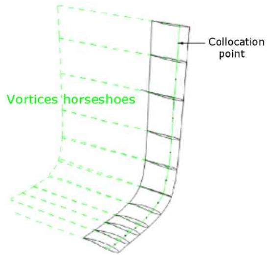
Figure 5: Vortex distribution along a wrap span
