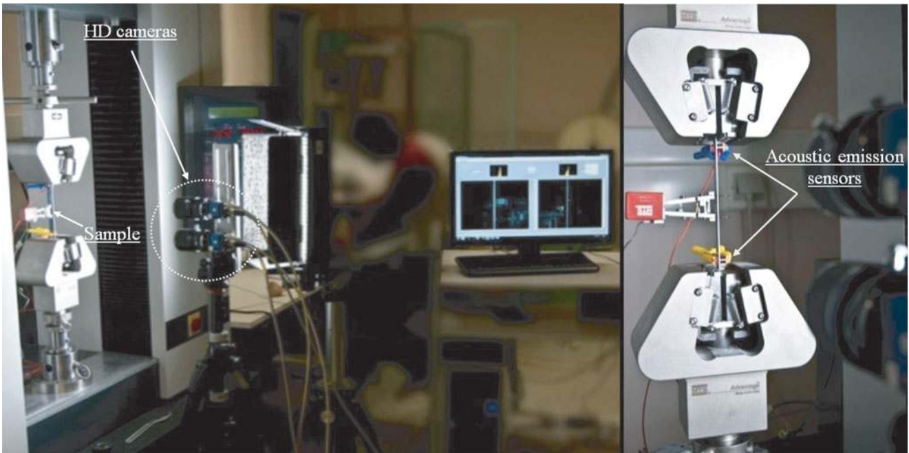
Fig. 1.2 Test set-up to measure intra-laminar tensile cracking by means of HD Cameras and Acoustic Emission technique
