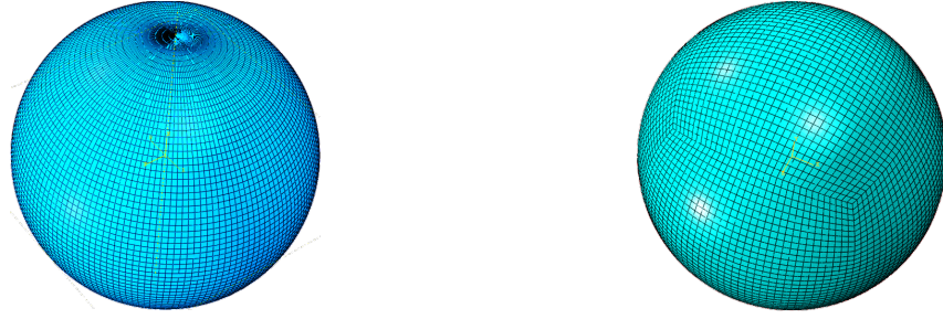
(a) Axisymmetric mesh with singular points
